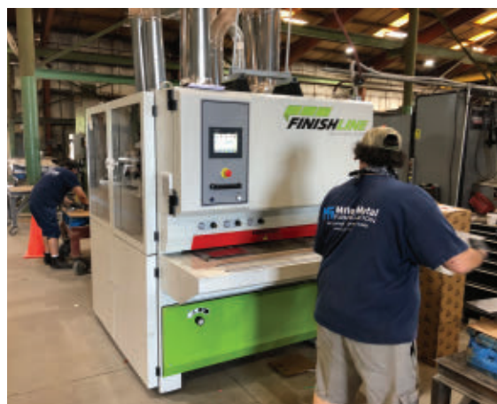
The FINISHLINE metal finishing machine proved to be a useful tool when it came to turning around laser-cut stainless steel parts that needed to have microburrs removed and edges rounded for a ventilator application.
