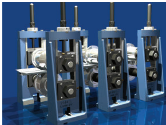
FIGURE 1 A roll form profile is formed through sets of roll tooling. Roll stands are removed to illustrate the workpiece transition.
