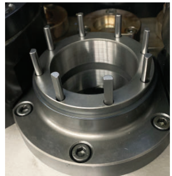
FIGURE 7 Inspect the tool's interior components, including the lifter pins, which should be straight and undamaged.
