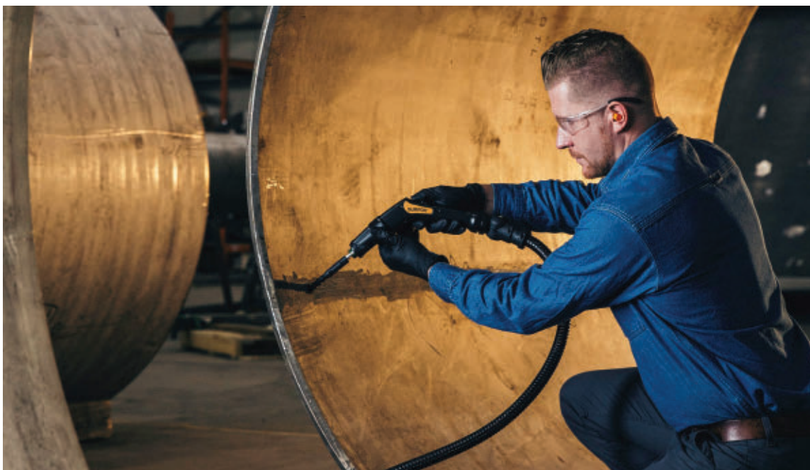
FIGURE 6 To ensure proper passivation, a technician electrochemically cleans a longitudinal weld seam in a rolled section of stainless steel.
