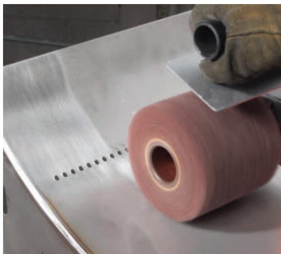
FIGURE 3 A nonwoven drum finishes a stainless steel surface. For effective finishing and optimal consumable life, different finishing media run at different RPMs.
