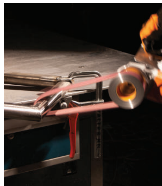
FIGURE 5 A belt sander puts the desired finish on a stainless steel tubular assembly.
