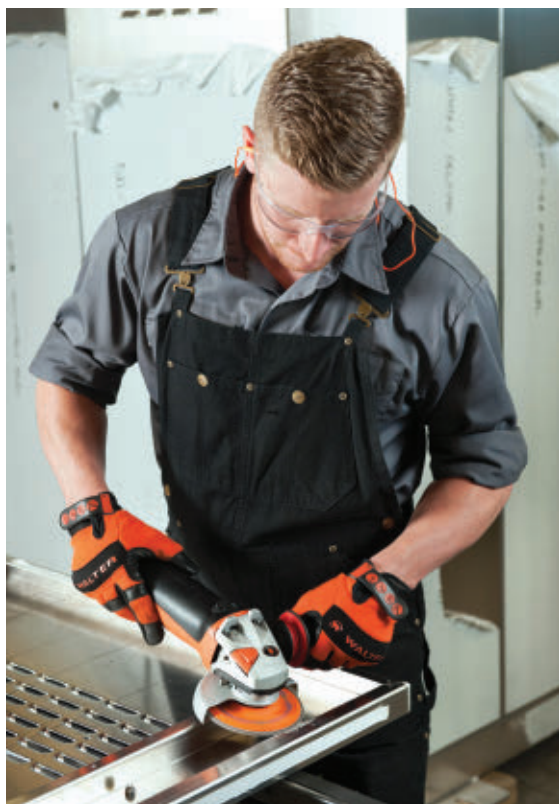
FIGURE 2 A worker finishes a stainless steel frame using a sanding disc.
