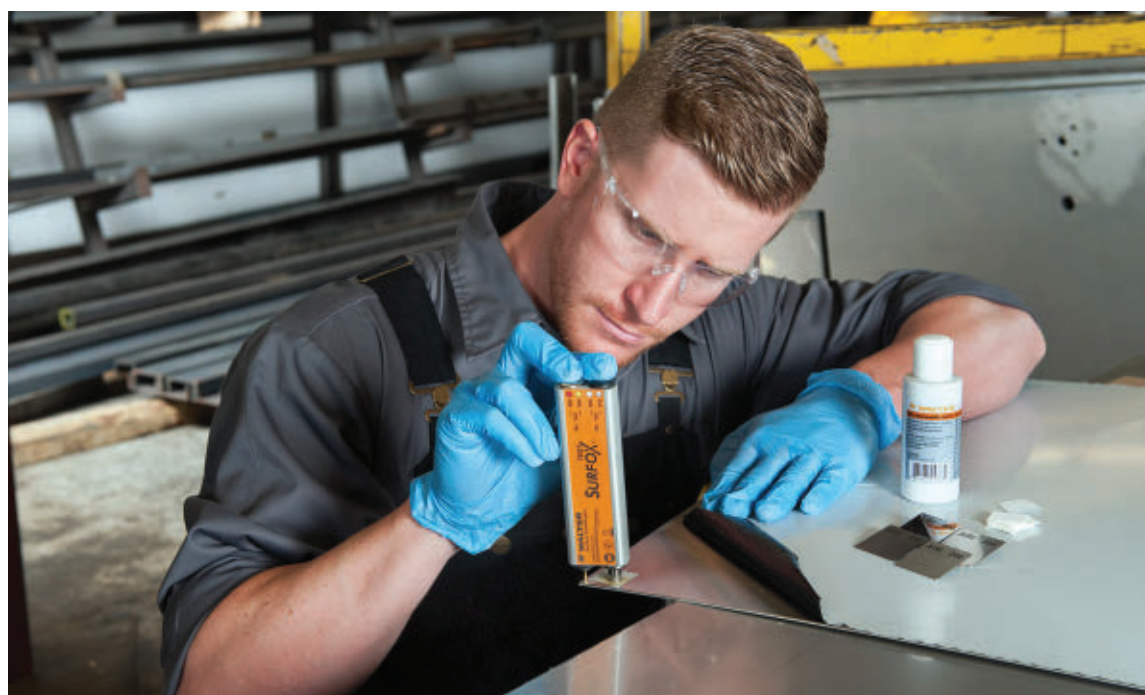
FIGURE 7 A stainless steel sheet is tested to ensure proper passivation.
