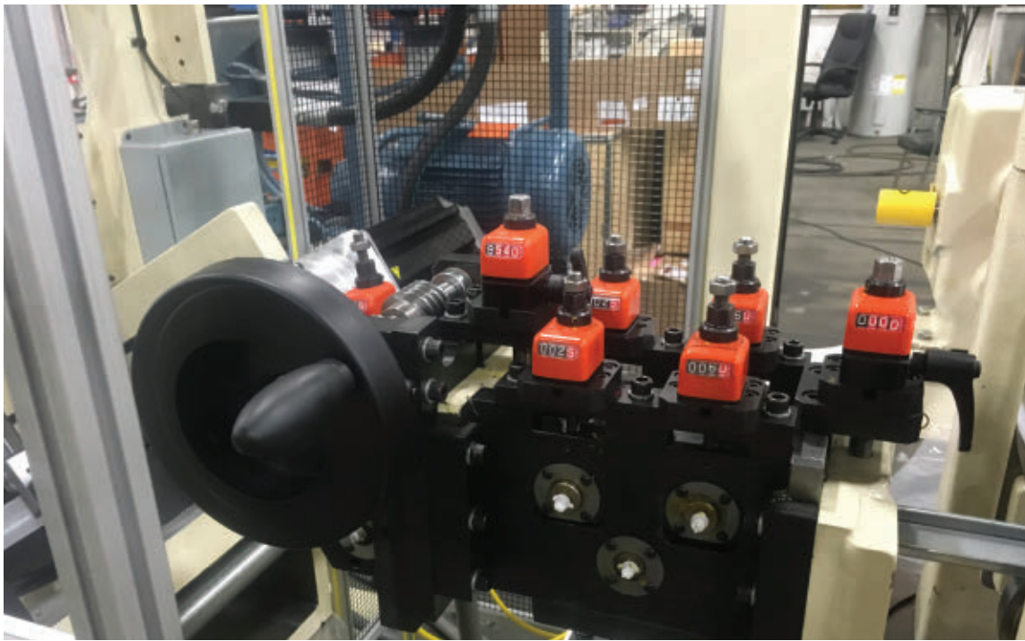
FIGURE 3 A sweep block uses a series of rolls and blocks to maintain straightness or put a desired curvature into a part.
