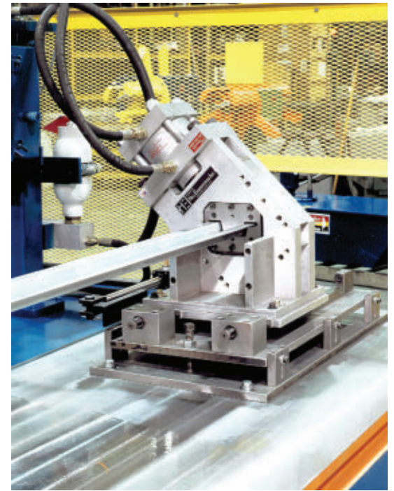
FIGURE 4 A cutoff die cuts roll formed parts to length as they exit the line.
