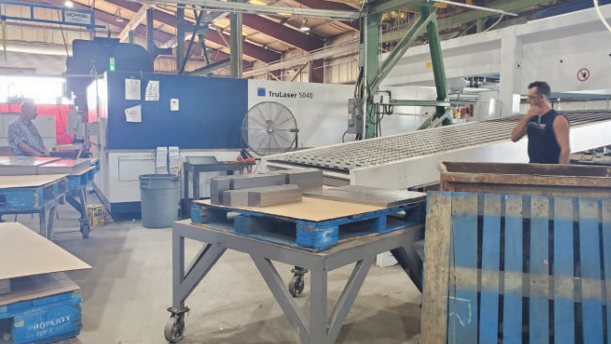
Miller Metal Fabrication's TRUMPF 10-kW TruLaser 5040 has added new laser cutting capacity for the fab shop.
