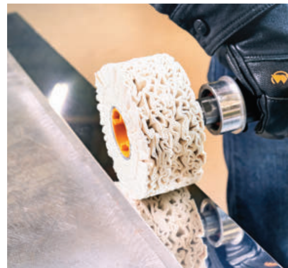
FIGURE 4 A polishing wheel creates a mirror finish on a stainless steel workpiece.
