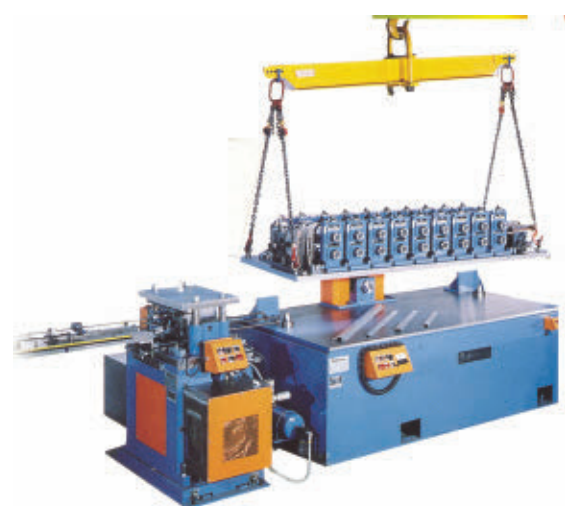
FIGURE 8 Designed for quick changeovers, rafted lines have pre-configured tool sets that can be lifted into place.
