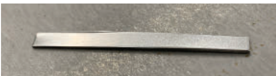
FIGURE 4 This slug was produced by the worn punch in Figure 3. Note the excessive rollover at the ends on opposite corners, tapering toward the middle.
